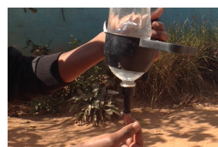
Image 19. One Way smell trap for shower (testing)
